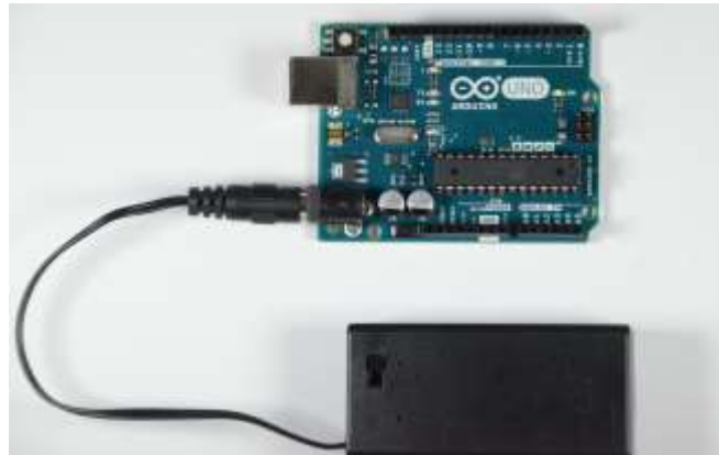
Figure 5, New Arduino pid 50 powered by a nine volt battery in a case
