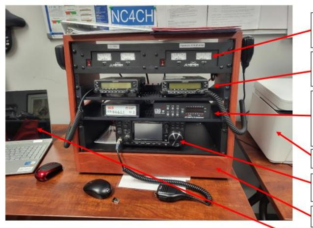
Dual rack-mounted power supplies. Left one powers the HF radio, modem, and tuner on the bottom 2 shelves. Right one powers the two dual-band radios in the middle.
