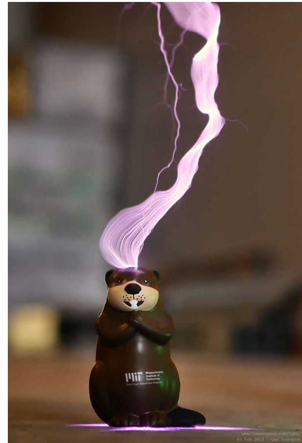
Parallel sparks from a modulated DRSSTC,
